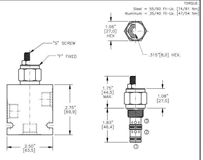
FOR ALUMINUM OR STEEL VALVE HOUSING CONFIGURATIONS SEE PAGE 0-032.1
