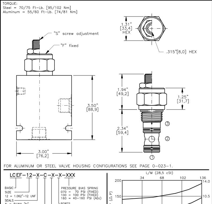
N = BUNA "N"DROP 0 = CARTRIDGE ONLY 04BX = G 1/2" BSPP 06BX = G 3/4" BSPP 10TX = SAE - #10 12TX = SAE - #12 V = VITON100 7.0 SPOOL-PRESSURE "C"=SPOOL (VENT TO OPEN) ADJUSTMENT-F = FIXED (FACTORY SET)
